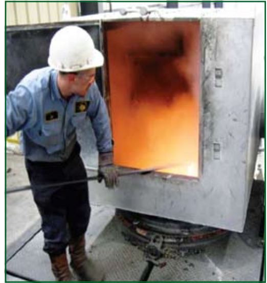
Melting furnaces operating at 2,300 degrees Fahrenheit.
