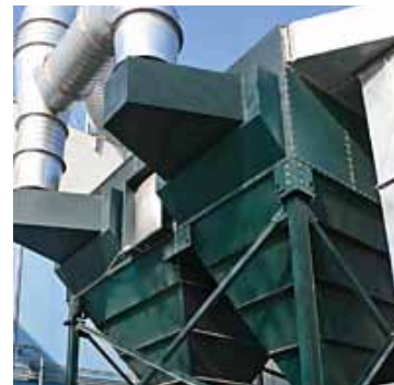
High Entry Inlet Cross flow is created through the filters. Eliminates upward “can” velocities associated with traditional hopper inlets.
