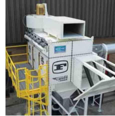
Top mount fan with premium efficiency motor, platform and ladder, silencer and explosion vent with blast deflector.
