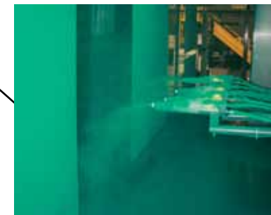
Individually Powder Coated Gold Series components are individually powder coated prior to assembly for superior corrosion resistance.
