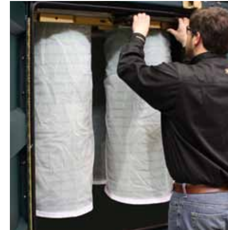
Overbag option for fibrous dusts like paper and fiberglass.
